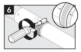
Verify the band clamp is positioned in the groove. Hand-tighten using screwdriver or nut driver until snug. Do not over-tighten to avoid damaging the clamp.
