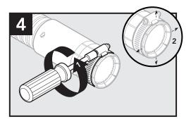
Loosen the band clamp to allow spreading of the split segments on the end of the coupler during insertion.
