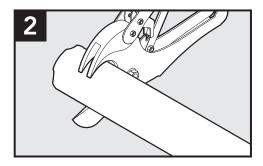
For the alternative conduit side, ensure your product has a clean, perpendicular cut.
