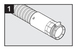
Use the PowerGuard Flex Coupler directions to properly install the corrugated pipe on the key lock side of the adapter.
