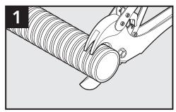
Ensure your conduit has a clean, perpendicular cut. Cut the duct at the top of the corrugation, rather than the dip, to enable proper alignment.
