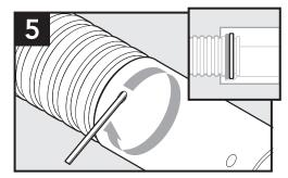
Following the arrow shape, insert the keylock strip into the pre-drilled hole. Push around the entire circumference, locking the corrugated grooves and coupler securely together. A water-based lubricant can aid in installation.
