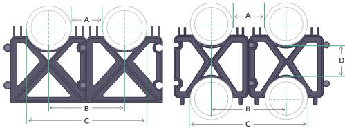
A: Between Conduit Horizontal (IN)B: Center to Center of Conduit (IN)C: Outside to Outside of Conduit (IN)
